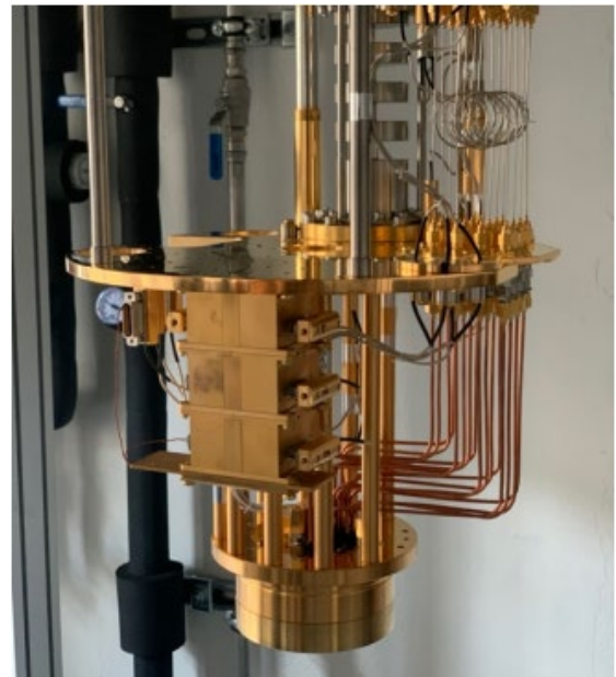
Three stacked MFT filter boxes under test in a cryo-free dilution fridge at University of Basel.
