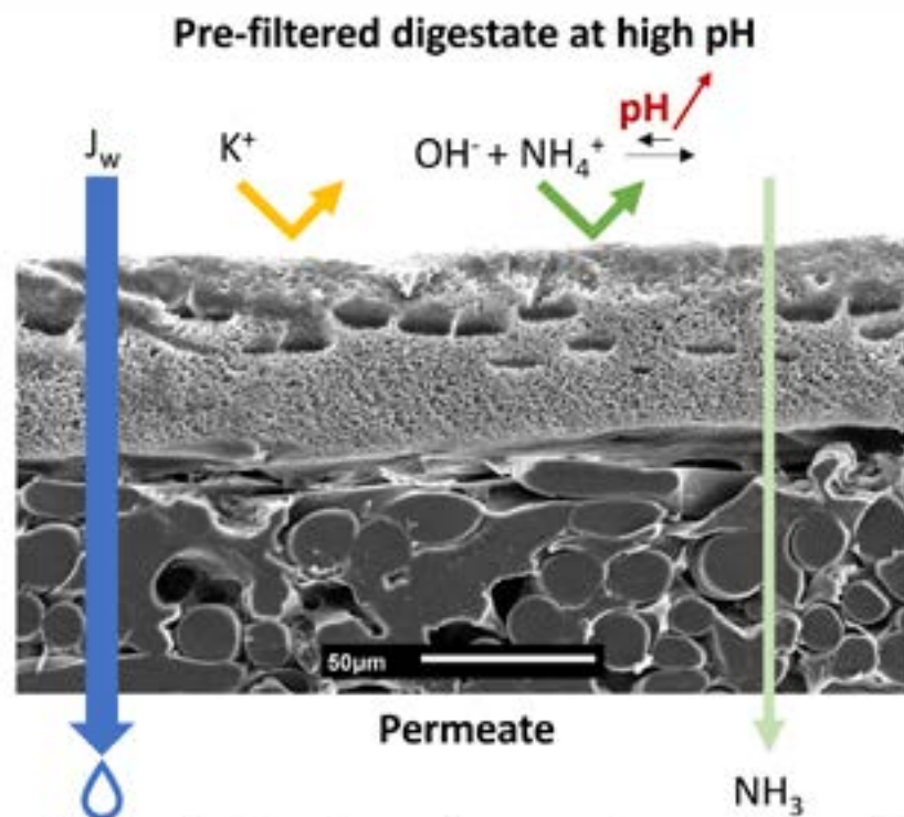
Figure 1: A schematic overview of the pH influence on the retention or permeation of potassium and nitrogen species through an NF or RO membrane.
