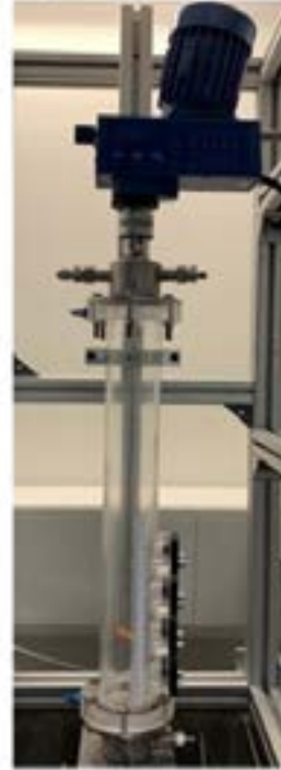
Figure 1: (a) Fused filament fabrication based 3D-printed stirrer with different properties, and (b) the experimental rig. Powder size is 7.5 \mu\text{m} and density is 1.9 \text{ g/cm}^3 .
