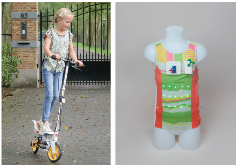
Figure 8. BRISH, wearable breathing trainer. A wearable supporting children to practise breathing training at home.
