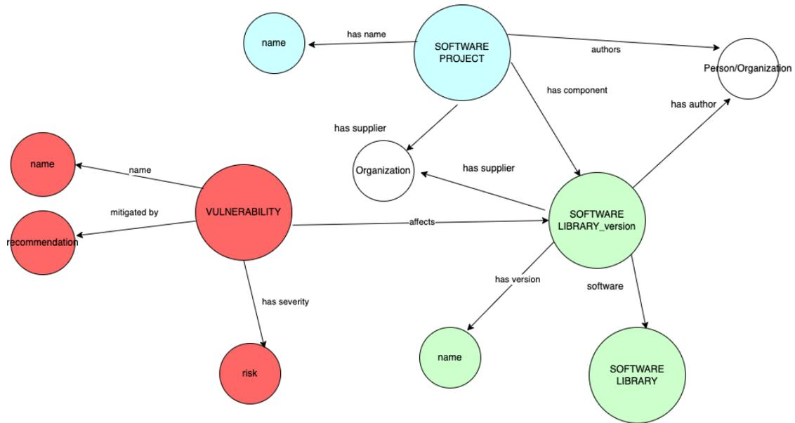
**Figure 2:** By relating vulnerabilities to software libraries and software libraries to software projects, a comprehensive picture of cybersecurity is obtained.
