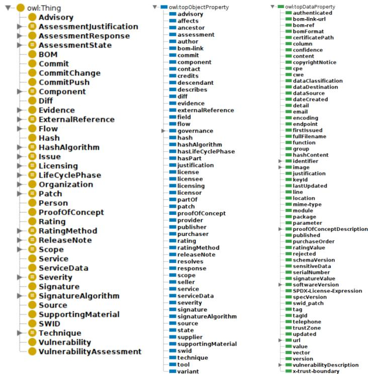
Figure 3: Main entities of CON: classes (left), object properties (center), data properties (right).
