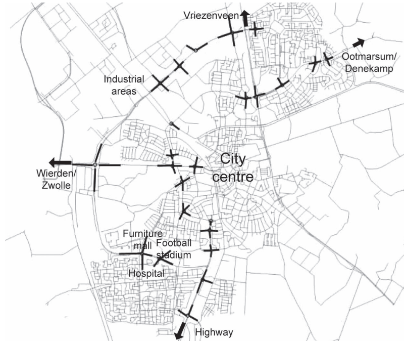
Fig. 1. City of Almelo, The Netherlands. The thick lines correspond with intersection links for which traffic data were collected.
