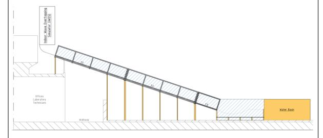
Within this thesis, you will conduct unique experiments to study the hydraulic loading from overtopping waves on the landward slope of a dike. The primary focus is to collect data on flow
