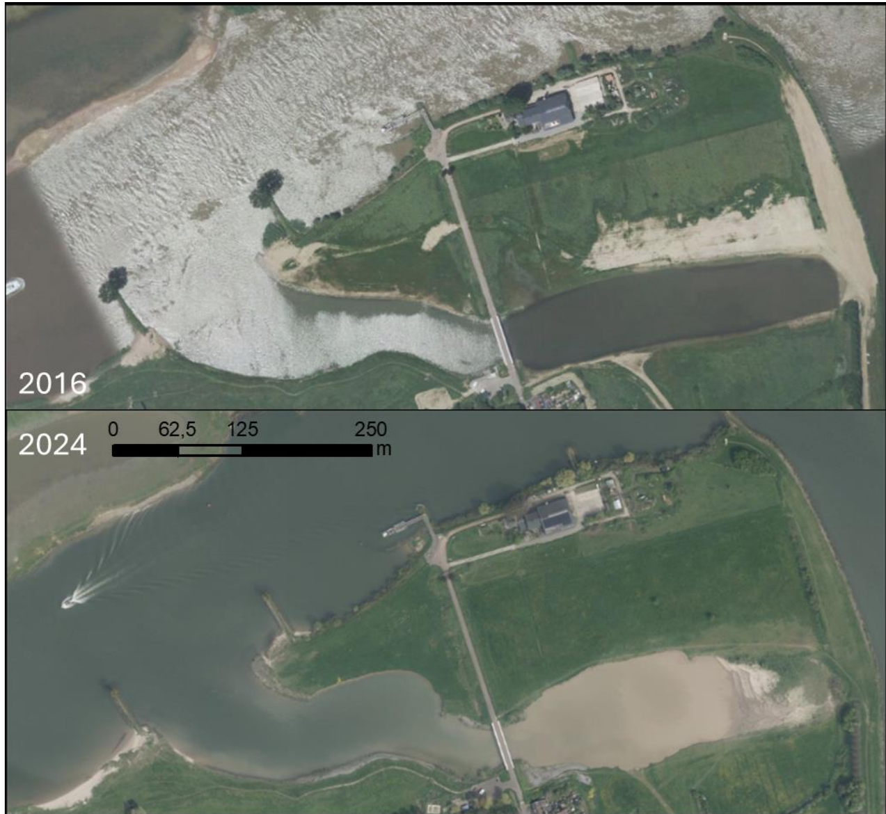
Figure 1: Example of bank erosion along a side channel of the Lek River
