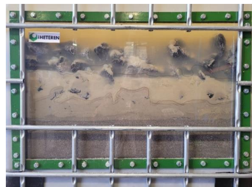
Figure 2: Large-scale experimental setup (1000-litre), ZBM applied on top of coarse surface
