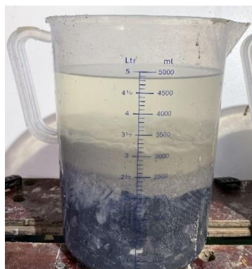
Figure 1: Small-scale experimental setup (5-litre), ZBM applied on top of sand surface
