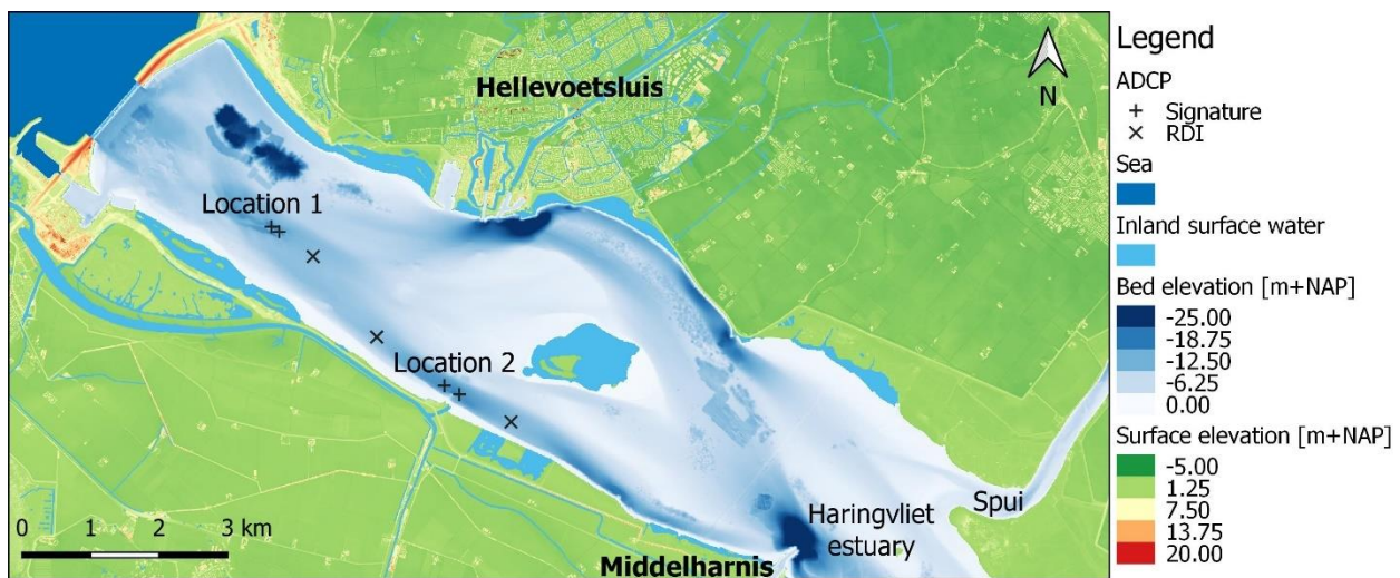
Figure 12: Positioning the ADCPs used on the bathymetry map of the Haringvliet estuary. Data layers from Rijkswaterstaat (2023a-b), Kadaster (2022) and Kadaster (2023)
