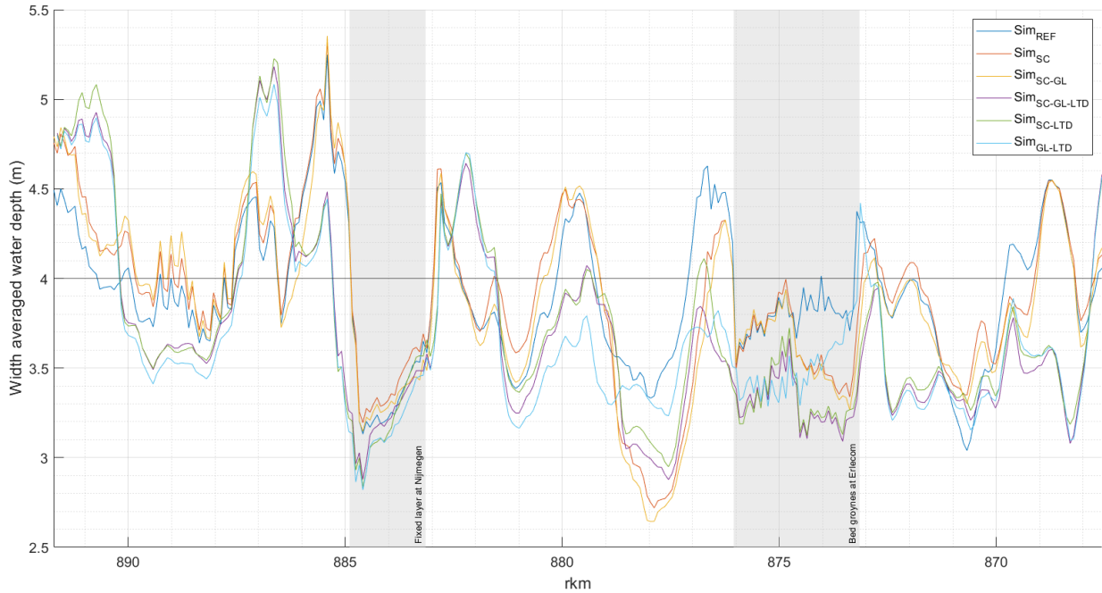
FIGURE 4.19: Width averaged water depth during OLA ( 1020 \text{ m}^3/\text{s} ) after 20 years along the Boven-Waal for the different simulations. The black horizontal line indicates a width averaged water depth of 4 meter that needs to be ensured (Rijkswaterstaat WVL, 2019).
