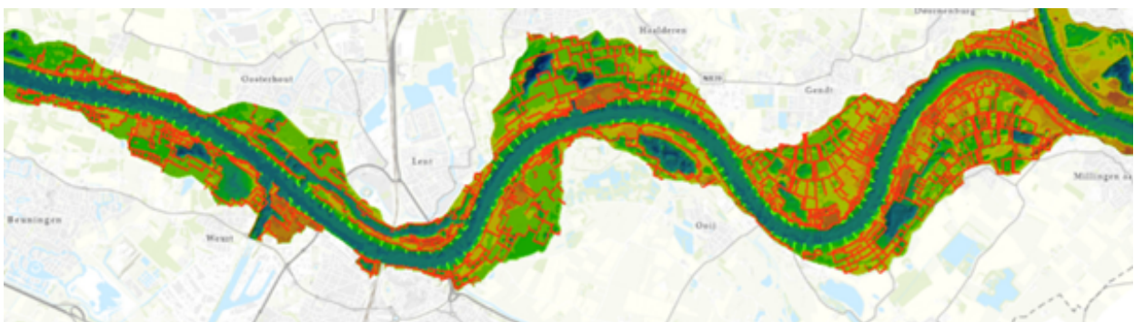
FIGURE D.4: The weirs that are changed for the lowering of groynes are shown in green. These weirs have been lowered to +1.20m OLR 2022. The weirs with a red colour have not been changed.
