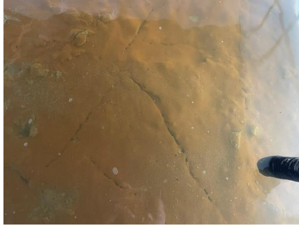
Figure 48, Large scale NaCl - Occurrence of cracks during emptying of the container
