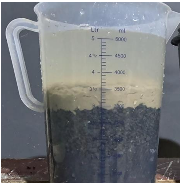
Figure 23, Small scale experiment coarse surface - Caldurite 2-8 mm before drainage
