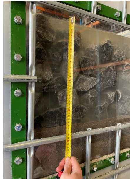
Figure 18, Large-scale experiment - Coarse surface layer build-up (35 cm)
