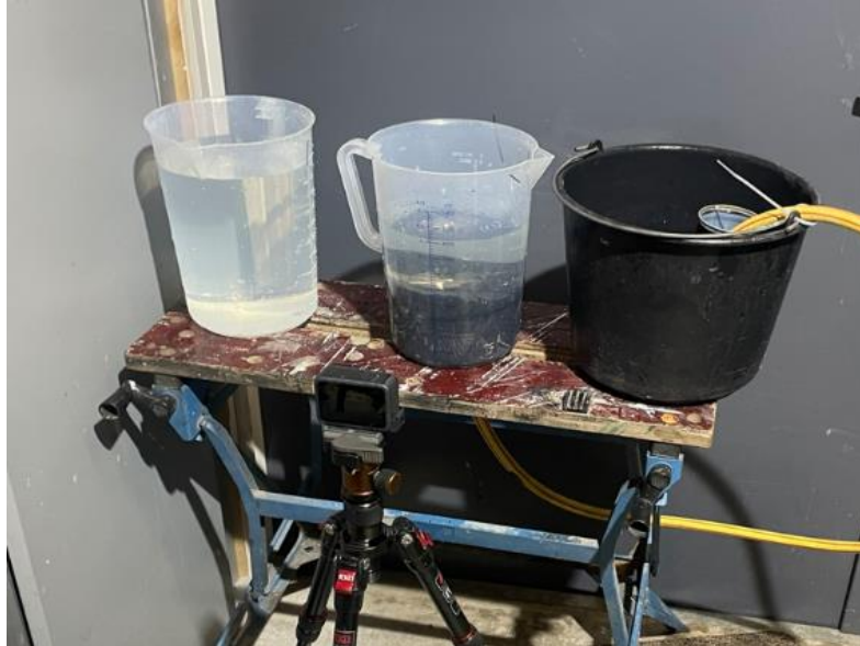
Figure 13, Small-scale experiment coarse surface – Experimental setup, second step, filling up the measuring cup up to the 4.5 litre indicator
