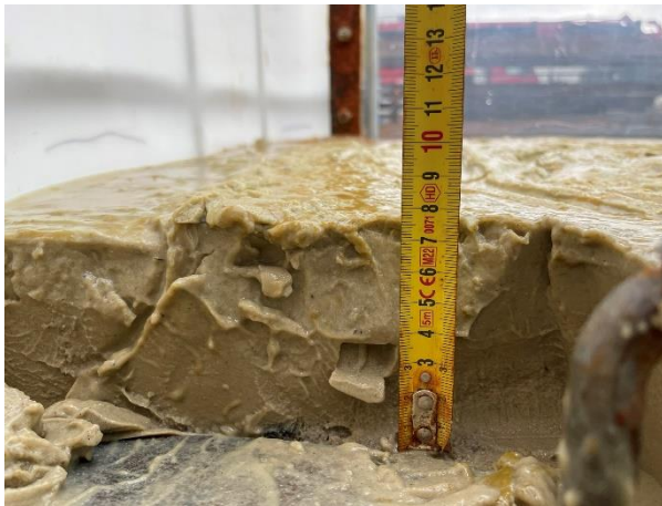
Figure 57, Large scale \text{CaCl}_2 - Cross section layer structure
