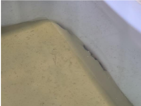
Figure 35, Large scale reference - Layer became loose on February 5 th
