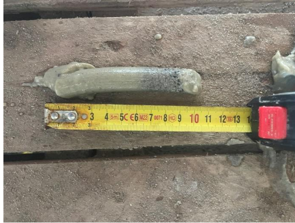
Figure 52, Large scale NaCl – Sample layer build-up
