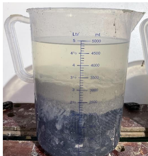
Figure 14, Small-scale experiment saline and lowered pH – Layer build up
