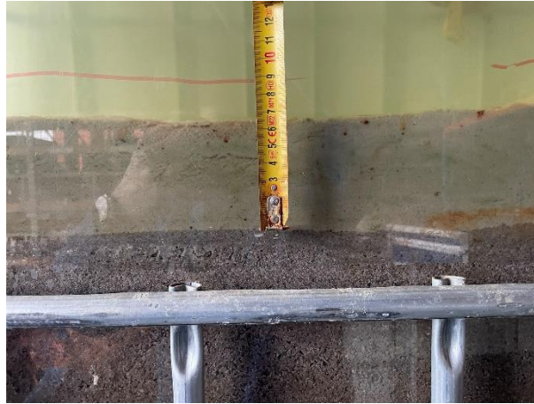
Figure 56, Large scale \text{CaCl}_2 - Layer thickness at day 21
