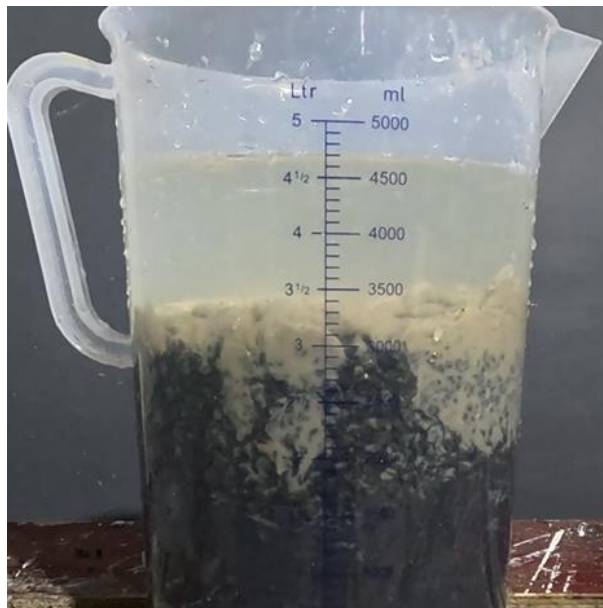
Figure 24, Small scale experiment coarse surface - Caldurite 2-8 mm after drainage
