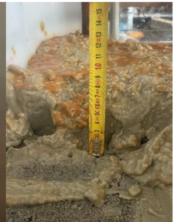
Figure 50, Large scale NaCl – Cross section layer structure
