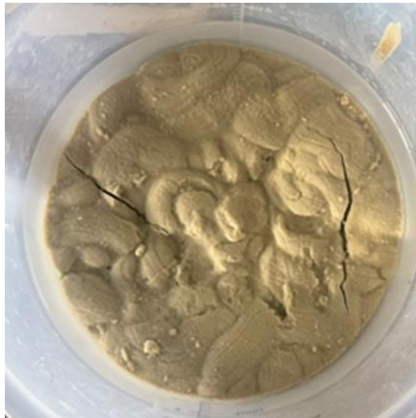
Figure 32, Small-scale experiment saline and lowered pH - Acidic water (pH 6.5) on day 4
