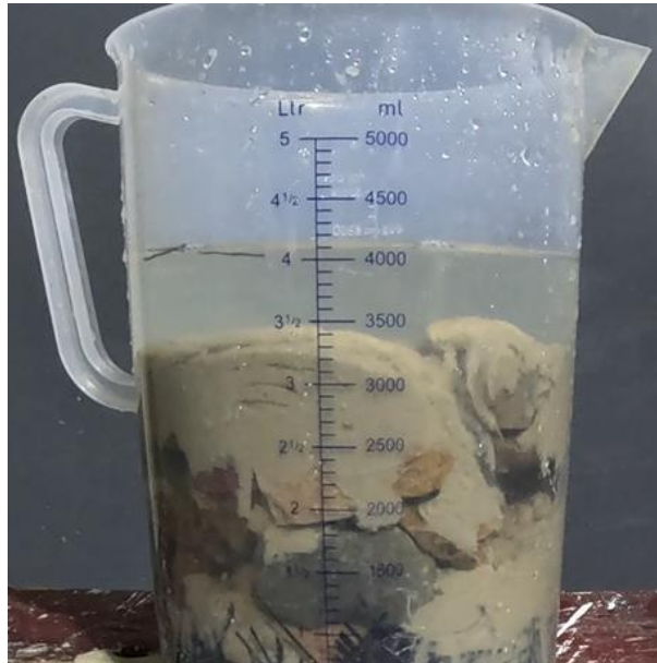
Figure 22, Small scale experiment coarse surface - Greywacke 11-56 mm after drainage
