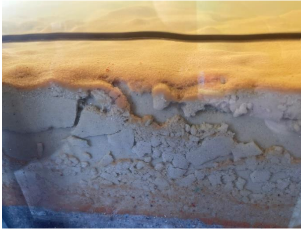
Figure 51, Large scale NaCl – Detachment ZBM layer from glass
