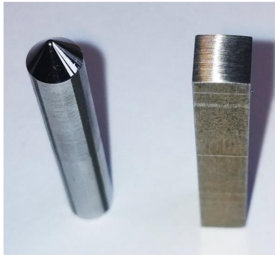
Figure 2: Pins used for the scratch tests (left) and reciprocating sliding tests (right).
