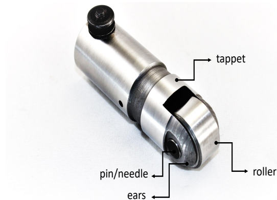
FIGURE 3: Example of a cam-roller follower unit.
