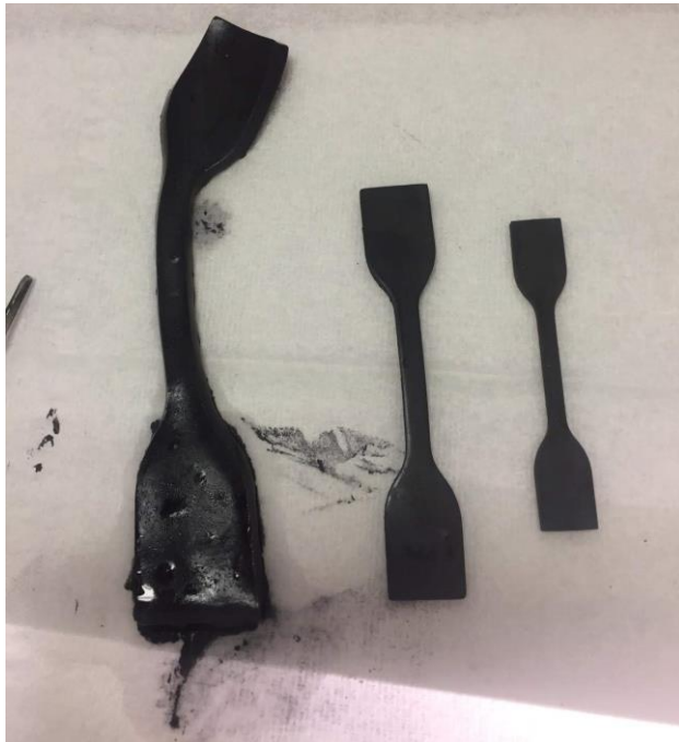
Figure 1-7. Severe swelling and blistering may result when a non-compatible elastomer/EAL pair is selected. The dumbbell-shaped specimens were initially of the same size.
