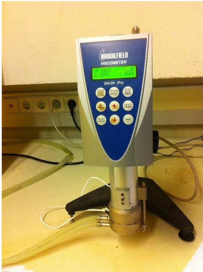
Figure 3-1. Viscometer used for measuring the viscosity at various temperatures at low shear rates.
