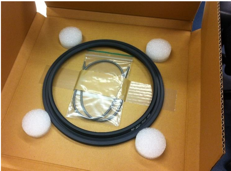
Figure 1-6. Package of 200 millimetres stern tube seal with its garter spring.
