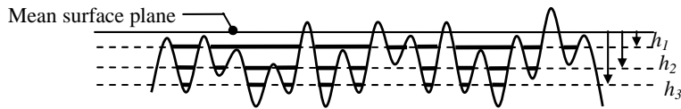
Fig. 2.4 Contact area in fully plastic contact (bold lines indicating real contact area at different separation levels).
