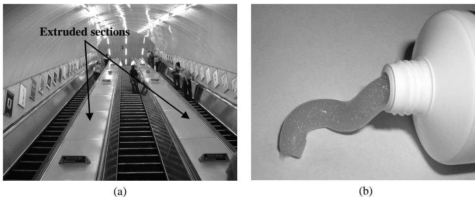
Fig.1.1 Examples of extrusion: (a) the escalator of London's "tube" system in which the handles are produced by extrusion; (b) a fleck of toothpaste is being extruded out of the tube.
